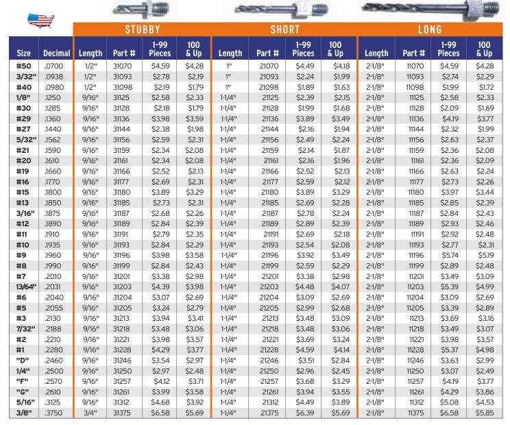
We are now stocking select diameter threaded drills in our new VERY STUBBY length. These Very Stubby Drills are intended for use in areas where space is severly limited. Overall length is only 3/8"! Feature industry standard 1/4-28 threads and like all of our threaded drill bits, they are made in the USA!
