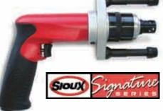
molded comfort grip and is designed for maximum operator comfort. 8-5/8" long, weighs just 2.7 lbs! Accepts industry standard 1/4-28 threaded rivet shaver bits (see page 14). "Shaving" depth is adjustable in increments of .001" for precise shaving of the rivet head without damaging the aircraft skin.
