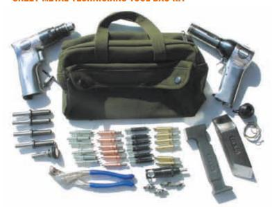
Great starter kit for aircraft sheet metal technicians, technical school students, or kit builders. Contains the necessary tools for most basic riveting, drilling, and countersinking applications.
