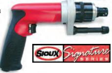
molded comfort grip and is designed for maximum operator comfort. 8-5/8" long, weighs just 2.7 lbs! Accepts industry standard 1/4-28 threaded rivet shaver bits (see page 14). "Shaving" depth is adjustable in increments of .001" for precise shaving of the rivet head without damaging the aircraft skin.
