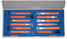
Contains #8, #10, & 1/4" Nutplate Jigs in Double Wing Style (Both Standard and Space Saver Spacing) and Single Wing Style (Also in both Standard and Space Saver Spacing).
